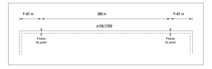
To calculate the number of prestressing elements required, the remainder of the run must be divided by Fe, see table on page 4.5.7.
