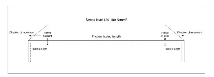
The calculations assume that the pipes are laid in sand in accordance with section 3 with a soil cover of max. 0.8 m and operating parameters of max. 16 bar and  $\Delta t$  max. 120°C.
