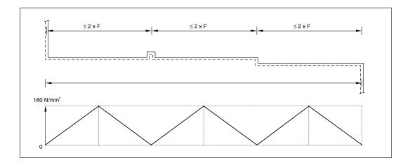
If a given section of pipeline exploiting natural changes in direction exceeds 2 x F, the section must be equipped with additional expansion zones and/or expansion components.
