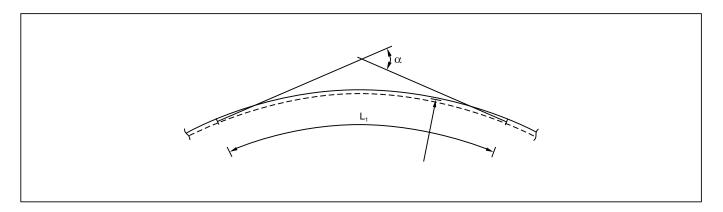
Permissible bending radius (min.) and bending angle (max.) in relation to pipe size.
