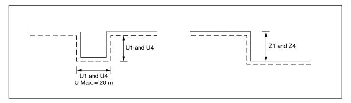
For laying method 1, 2 or 3, use U1 and Z1. For laying method 4, use U4 and Z4.
