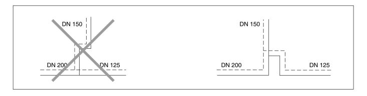
If more than two dimension changes are required, the following minimum "reduction lengths" (R<sub>i</sub>) between two successive reducers must be observed.
