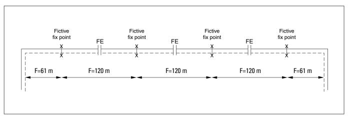
Prestressing length  $F_m = (90 - 10) \times 120 \times 0.005 = 48 \text{ mm}$
